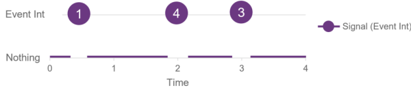
Figure 3. An example of a Signal that yields nothing or an Event containing a value of type Int .
