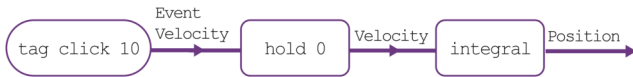
Figure 7. Visualization of positionSF transforming the event stream to the position signal. Note that click is of type Event() .
