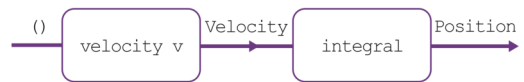
Figure 6. Visualization of positionSF . The arrow represents the signal that is modified by the signal functions velocity and integral .
