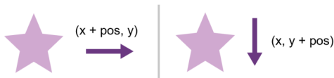
Figure 4. Animation of a star depending on the position pos . The direction is determined by the definition of the coordinates in the GUI. E.g. the coordinates on the left correspond to a movement along the x-axis, whereas those on the right result in a movement along the y-axis.
