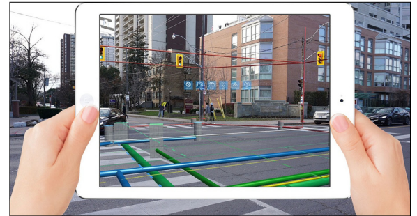
Screenshot of the web-app with an educational model on the OST campus Rapperswil displaying different types of pipes Own presentation
