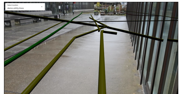
Screenshot from Stäfa showing waste water pipes; the manholes seem to be above the ground, but it's an optical illusion Own presentation
