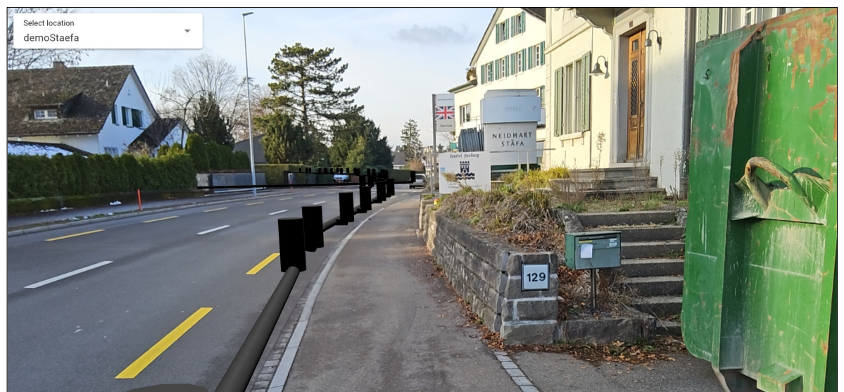
Screenshot from Stäfa showing waste water pipes; the manholes seem to be above the ground, but it's an optical illusion Own presentation
