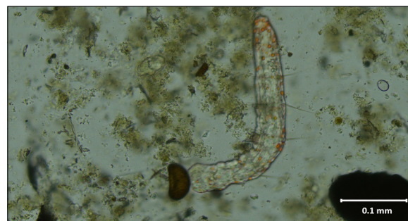
The image of the foulants after ~25 days with dosed small-sized 0.1 g/L microplastics in wastewater under a microscope Own presentation
