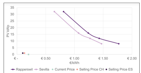
Price necessary for electricity for an economically feasible hydrogen microgrid Own presentment
