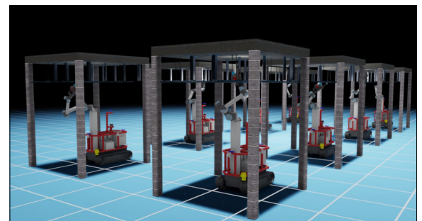
Massive parallel training within NVIDIA Isaac Gym as enabler for training RL-policies in complex environments. Own presentation
