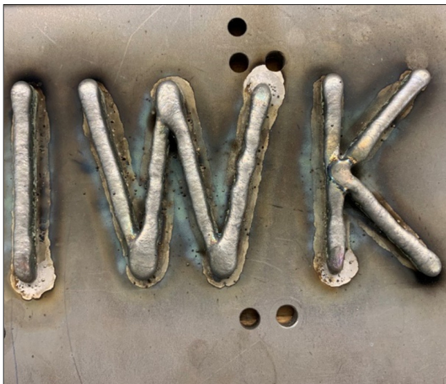
side and top view of demonstrator, NiCr22Mo9Nb deposited onto DC04 mild steel plate Own presentation
