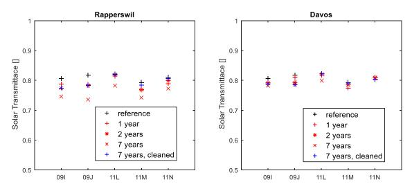
Figure 5: Solar transmittance of all tested AR-coated glass samples after different periods of outdoor exposure in Rapperswil.
