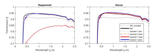
Figure 4: Solar transmittance of all tested AR-coated glass samples after different periods of outdoor exposure in Rapperswil.
