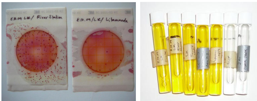
Fig. 13: Two different methods to determine the water-quality in the field. The left picture shows a test-result from 3M-Petrifilm (E.coli/Coliform Count Plate) and the right picture shows a presence/absence-test with Colilert by IDEXX (also E.Coli / Coliform). Both methods are easy to handle in the field because no additional equipment is required. The results are ready after an incubation time of 24 hours.
