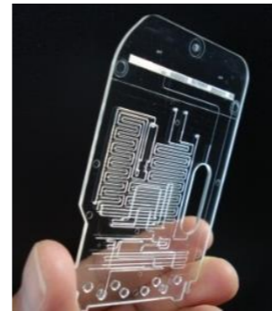
Microfluidics features 50\text{-}100\ \mu\text{m}
