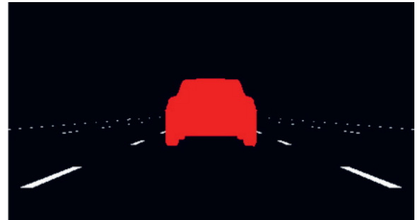
How the follower perceives the leader car through its camera Own presentment
