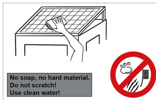
Figure 23: Instructions for cleaning the solar panel
