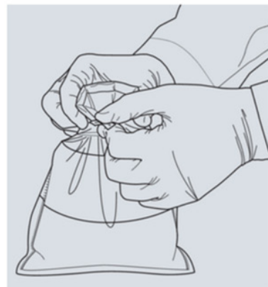
6. Bring the two wire ends together and twist tie them
