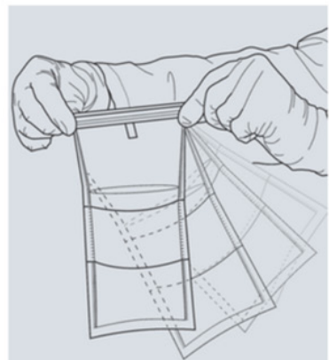
5. Hold the bag by the wire ends and whirl it 3 - 4 times to make a seal.
