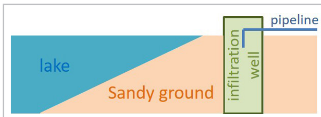
Figure 16: Scheme of an infiltration well
