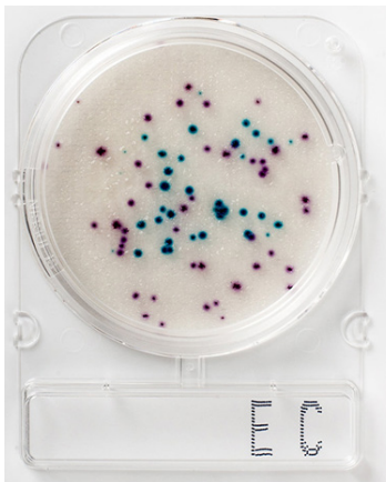
Figure 55: EC dry plate. Dots indicate CFUs. Blue = E. coli, purple = total coliforms
