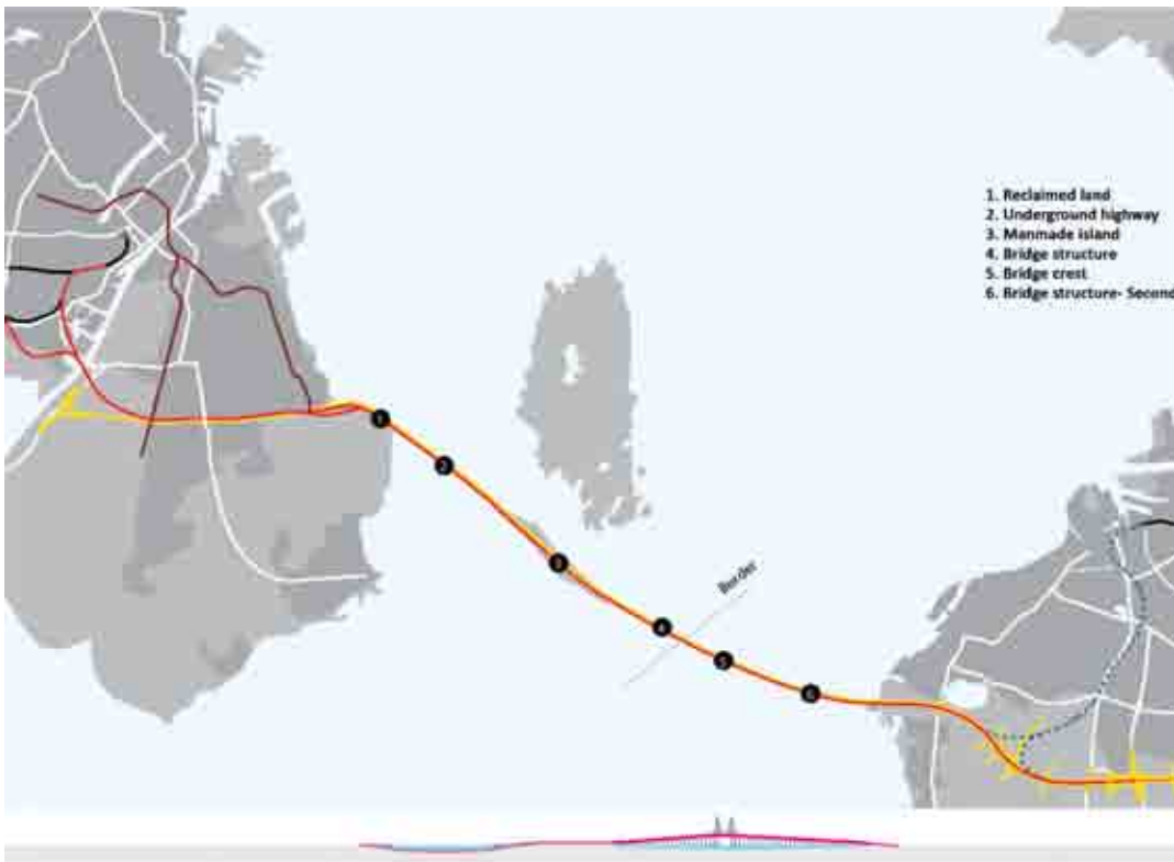
FIGURE 4. The complete landscape design of the Oresund Bridge. The design has six parts: Two landings on each side, the manmade island in the middle, the bridge and its crest and the tunnel structure.
