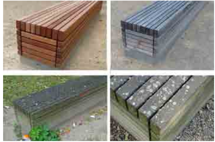
FIGURE 2. Change to wooden bench in full shade under a tree canopy over 7 years. Above: Year of completion and 1 year later. Below: 7 years after completion.
