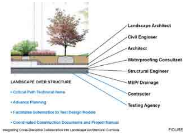
FIGURE 1. Landscape over structure construction detail
